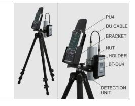
4) Use **DU cable** for connecting detection units to BT-DU4
